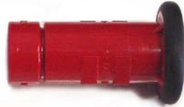
#91.1030 nozzle, adjustable from (A) closed/open, (B) to fog, (C) to straight stream. Nozzle from red polycarbonate with bumper, steel inner stem. For use up to 100 psi @ 8 Gallon per minute. Nozzles from other materials available.
